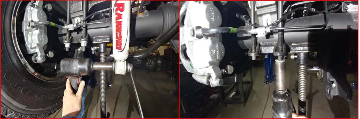
Remove the rear shocks. Support the axle with a suitable jack. Loosen but do not remove the driver side u-bolts. Remove the passenger side u-bolts completely and lower the axle.
