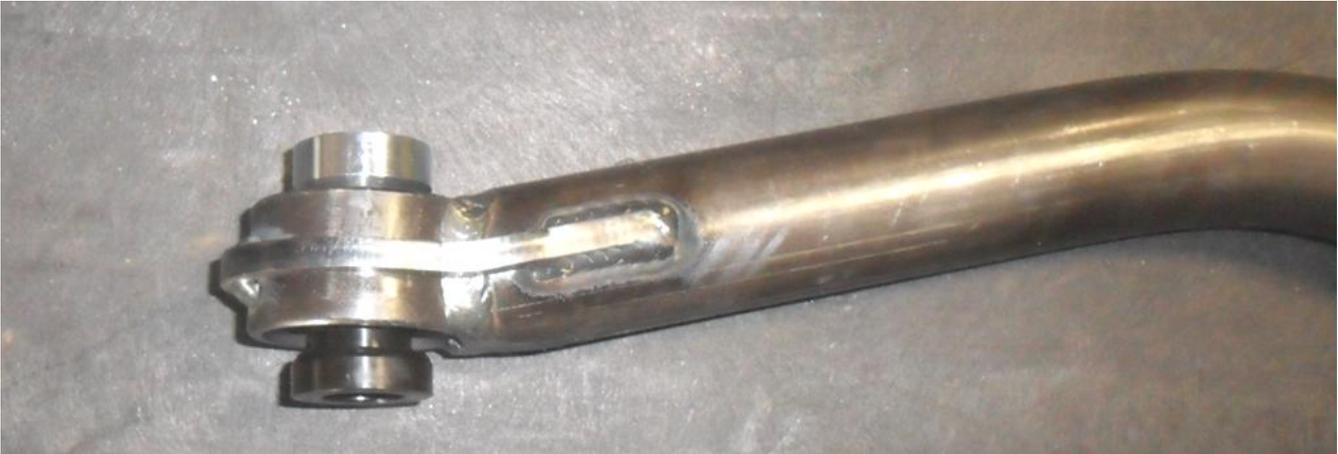
11. Slide the assembly into the frame side bracket and install 18mm, factory bolt and nut to secure the uniball.
